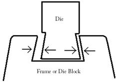
Make sure these two angles are the same for maximum contact. Also check the corner radius for interference.
